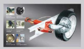
Overrun Device: The control unit for the automatic overrunning system. Once a certain threshold is reached, it transfers the thrust to the brake rod through a bell crank which in turn activates the wheel brakes with a Bowden cable. AL-KO braking system overrun devices far outstrip the legal requirements in brake tests.
